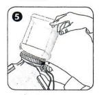
Twist reusable reservoir onto lid that is attached to the top of trap.
