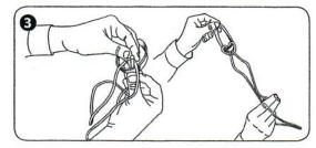
Place middle point of orange twine just behind the front of the white wristlet. Grab the ends of orange twine and loop through edge of wristlet and then through loop in orange twine.
