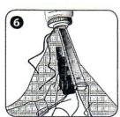
Attach trap to tree (about chest level) by drilling drywall screw through the middle point of 18" cedar strip.
