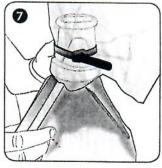
Place resealable black cable tie around replaceable bag and cylinder and pull until taut.
