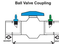
GLUE IN COUPLING WITH FLOW ARROW POINTING IN THE DIRECTION OF THE WATER FLOW
