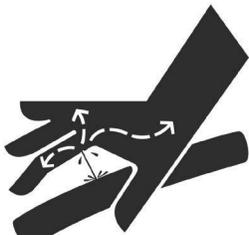
Escaping fluid under pressure may penetrate the skin causing serious injury. Avoid the hazard by relieving pressure before disconnecting hydraulic lines. Tighten all connections before applying pressure and inspect hoses regularly for wear or damage. If an accident occurs, see a doctor immediately. Any fluid injected into the skin must be surgically removed within a few hours or gangrene may result.
