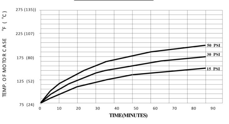
THIS GRAPH IS FOR USE AS A DESIGN GUIDE. IT IS BASED ON RUNNING CONTINUOUSLY WITH AN AMBIENT TEMPERATURE OF 75° FINSTILL AIR.
