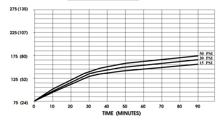
THIS GRAPH IS FOR USE AS A DESIGN GUIDE. IT IS BASED ON RUNNING CONTINUOUSLY WITH AN AMBIENT TEMPERATURE OF 75°F IN STILL AIR. THE THERMAL BREAKER WILL OPEN WHEN THE CASE TEMPERATURE REACHES 280°F.
