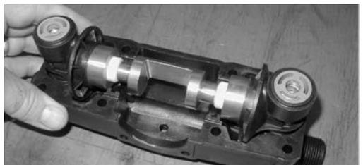
**Diaphragm/Valve Casing Assembly: (Fig. 5)**
