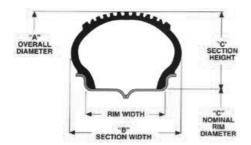
The first number on the tire size refers to the diameter of the tire (except fot the 280, 400, 410, and 480 tires). For instance, if the tire size measures 9-350-4, then the tire's overall diameter is 9". The second number refers to the section or overall width, and the third number refers to the diameter of the rim (all measured in inches).
