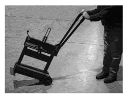
Easy to Transport. To transport unit, open handle to full open position. Insert support pin through holes at the end of the handle to lock handle in open position.
