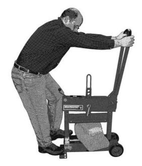
Place material to be cut in the center of the base. Lower tip blade by turning crank handle clockwise and lower handle until it rests at a 45 ° angle to base.
