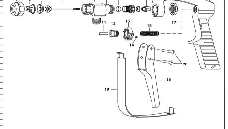
AB23H-Kit-Spare Parts Kit (For Brass, Nickel Plated GunJet Spray Gun) Includes all items marked with \* AB23H-SS-Kit-Spare Parts Kit (For Stainless Steel GunJet Spray Gun) Includes all items marked with \*
