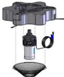
The motor unit attaches using stainless steel hardware. 3 section, U.V. resistant, high density thermo-plastic float. Bottom screen to protect the unit from debris.
