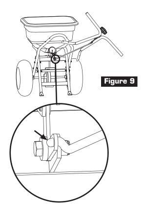
9. Turn Handle Assembly sideways and install Linkage into Rate Gate Lever as shown in Figure 9.
