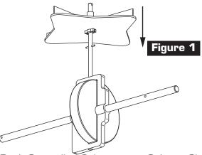
1. Push Spreading Spinner onto Spinner Shaft as shown in Figure 1. Make sure Roll Pin in Spinner Shaft engages with slot in Spinner.
