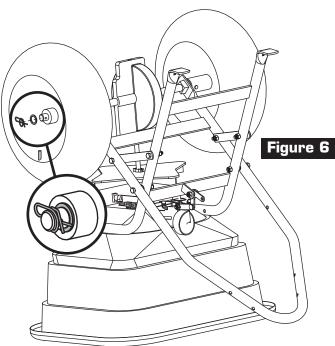
6. Install Wheel on the opposite side of the Axle (valve stem out) until it touches Axle Bearing and Washer.
