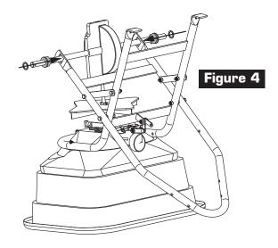
4. Install both Axle Bearings into the square holes as shown in Figure 4.
