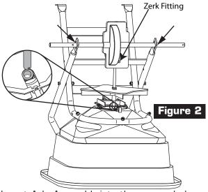
2. Insert Axle Assembly into the square holes on the Axle Support as shown in Figure 2.
