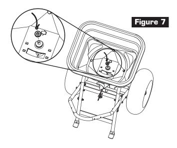
7. Inside the hopper, assemble the Felt Washer and Agitator Wire onto the Spinner Shaft as shown in Figure 7.
