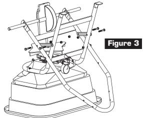
3. Align the Cross Braces to the Hopper and Axle Supports as shown in Figure 3. Using (4) 1-1/2" Bolts and Nylon Locknuts, assemble Cross Braces. Tighten Cross Brace Bolts securely.
