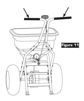
11. Install Handle Grips on Handles of Spreader as shown in Figure 11.
