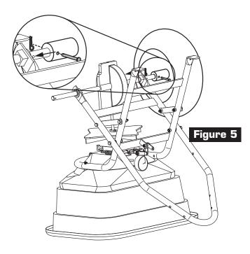
5. Locate the hole on Axle closest to the Axle Bearing and Washer.
